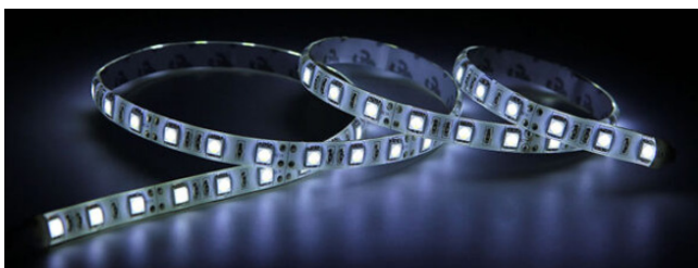
Figure 1: LED light strips consist of narrow, flexible circuit boards populated with surface-mount LEDs of various colors. With a built-in IC, individual RGB LEDs on the light strip will be independently addressable.
