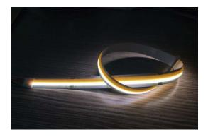
**COB LED light strips:** In chip on board (COB) light strips, the unpackaged LED chips are mounted on a thermally efficient substrate placed below a uniform phosophor coating. The approach supports a much higher packing density. COB light strips produce consistent output along their length, eliminating hotspots and generating up to 1200 lm/m.
