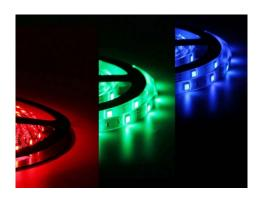
**LED light strips:** LED light strips consist of narrow (8 to 10 mm), flexible circuit boards populated with surface-mount LEDs and the associated drive circuitry. The LEDs can be monochromatic or multicolor, including RGB triads or RGBW chips. With the addition of a built-in IC, each LED on a light strip can be individually addressed and software controlled, making it possible to add dramatic accents to even the smallest spaces. LED density can be customized for the application.
