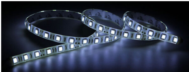
Figure 1: LED light strips, consist of long, thin, flexible circuit boards populated with surface mount LEDs and driver circuitry.
